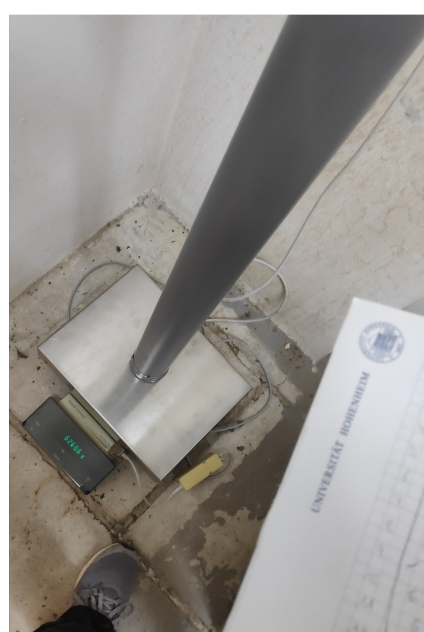
2. Filling of tubes to standardized weight, monitoring of water content
