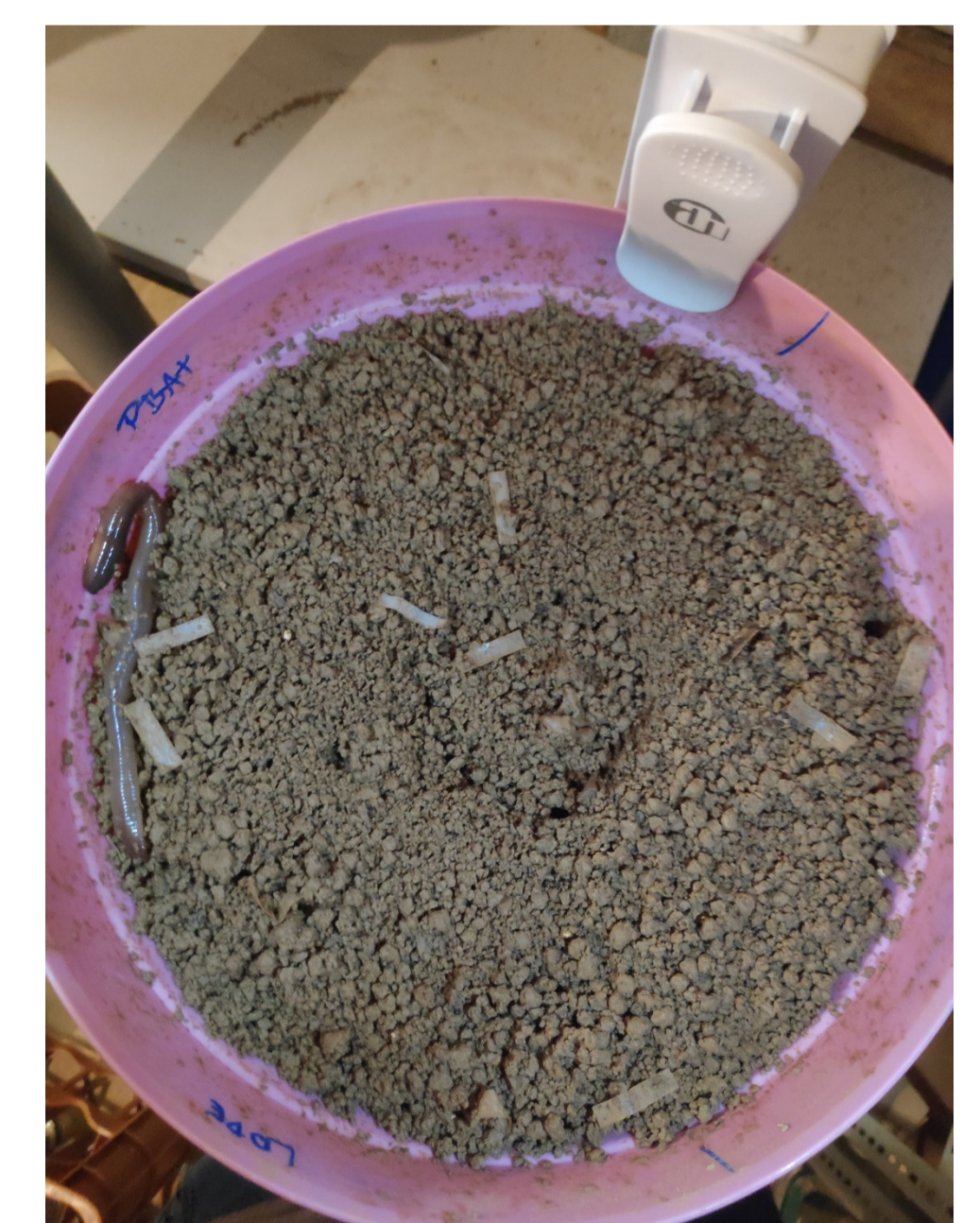
Plastic strips remaining on the soils surface after two days.
