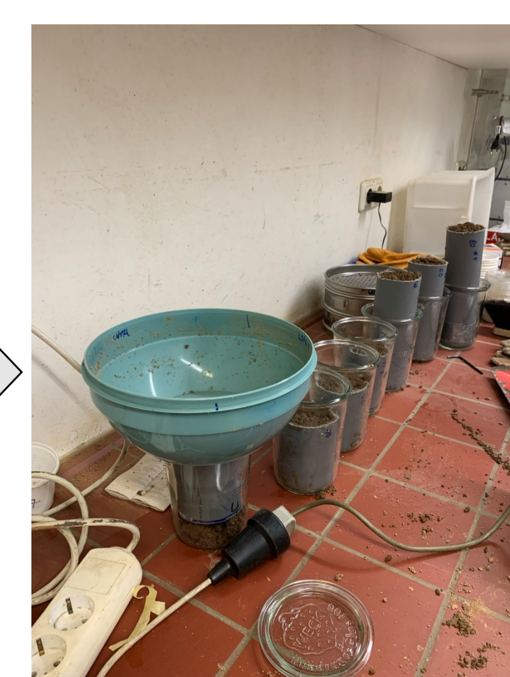
2. Sectioning of tube and sieving of each section
