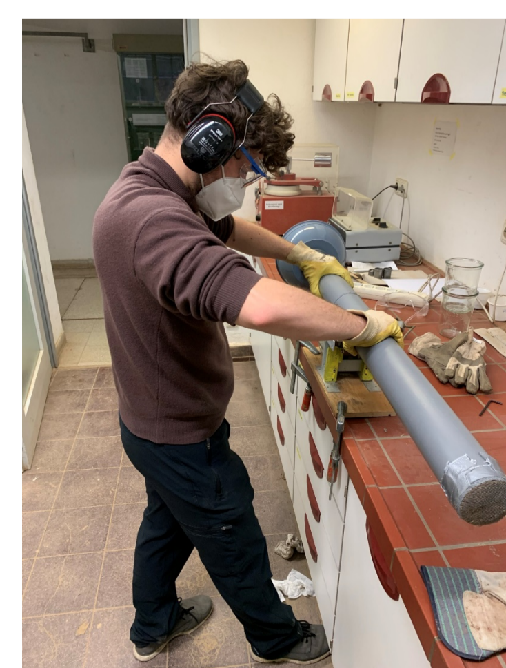
1. Opening of PVC tubes with a table mounted circular saw
